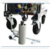
Tensioning wedges allow quick and easy pump exchange.
